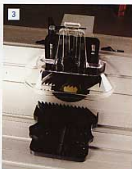
The guard plus the vertical and horizontal pressure fingers in place
