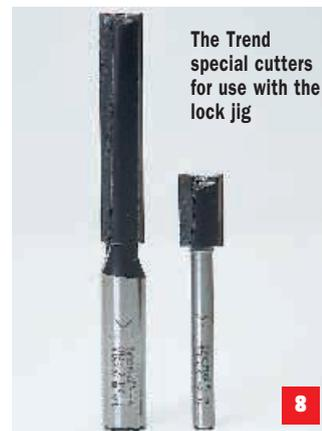
The Trend special cutters for use with the lock jig
