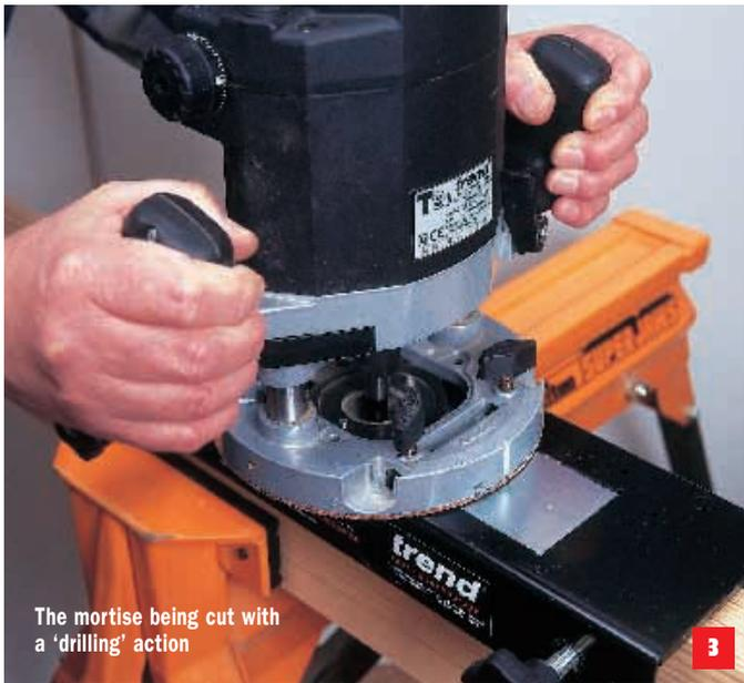
The mortise being cut with a 'drilling' action
