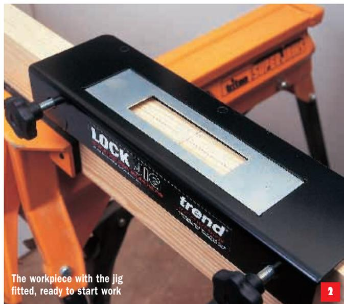
The workpiece with the jig fitted, ready to start work
