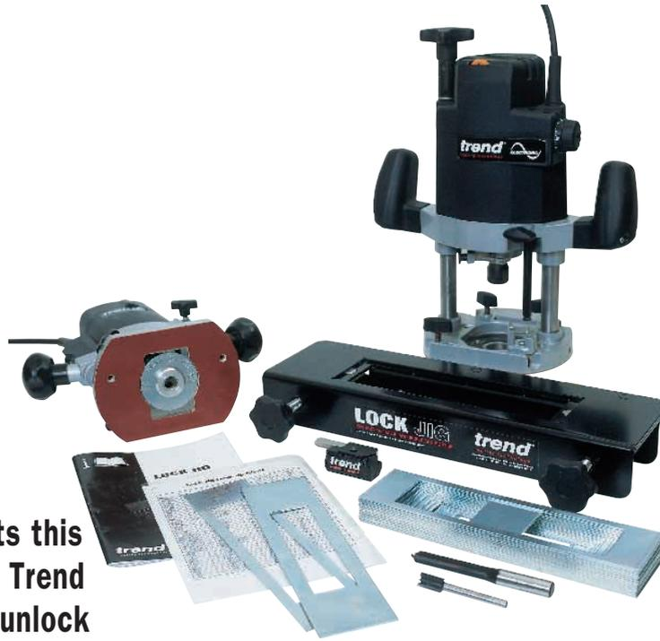
This new jig from Trend is designed to make short work of fitting door locks. By means of a set of interchangeable templates and with a router fitted with a 30mm guide bush it enables the mortise and face plate recess for most popular makes of lock to be cut quickly, easily and accurately. Photo 1 shows the components of the jig.
