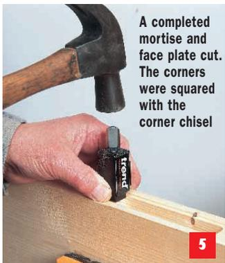
A completed mortise and face plate cut. The corners were squared with the corner chisel
