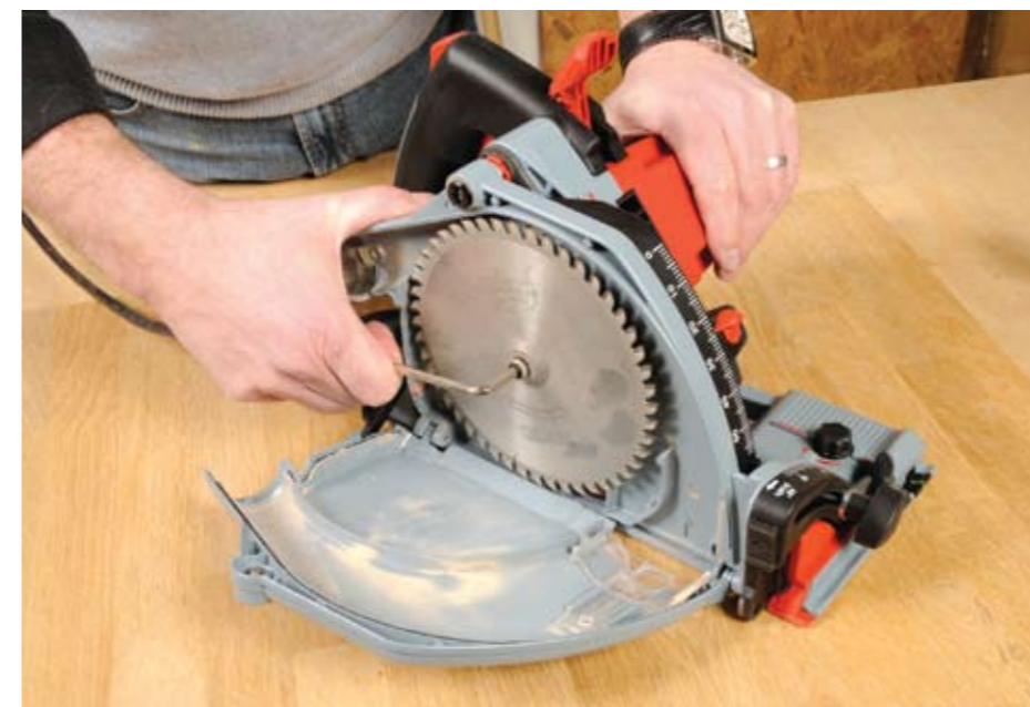
It took literally seconds to change between the two included blades, with no danger to the user and a snap in, snap out approach that won't hinder the worker under pressure
