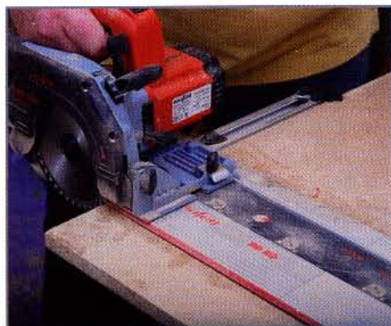
Using the long alloy guide; note the protractor at the end for setting angles of cut
