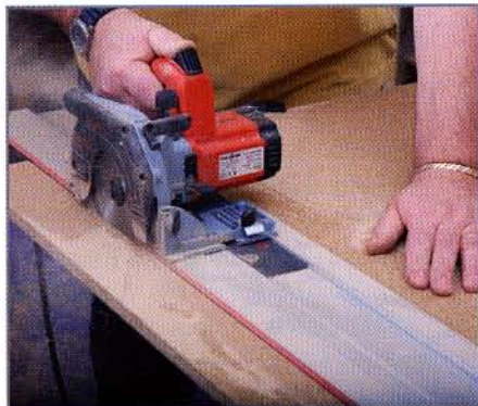
No dust extraction is available, but the saw glides down the guide very easily using only one hand
