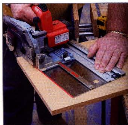
Starting a cut using the crosscut guide; note that the cut is angled, having been set by the screw on the left
