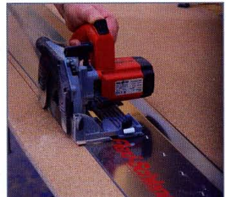
Nearing the end of a cut using the Flex guide which is dead easy to use
