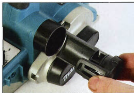
Dust can be extracted from either side
