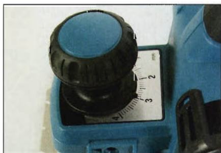
The maximum depth of cut is 4mm
