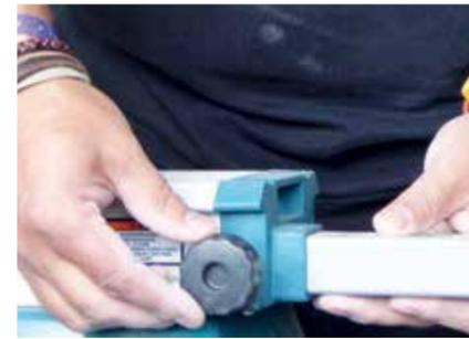
▲ A second extension arm has the roller, which allows work to be easily moved across the stand
