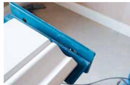
▲ It allows any work to butt up against it for fast repeat cuts
