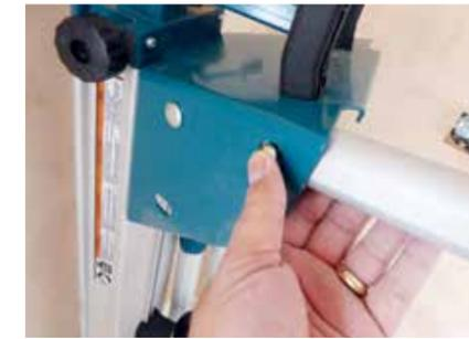
▲ Depressing this button allows the legs to be opened or closed
