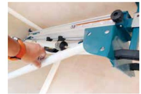
▲ The pins are sprung to lock open or closed for easy deployment
