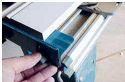
▲ A simple stop on the extension arm can be engaged by sliding it upwards
