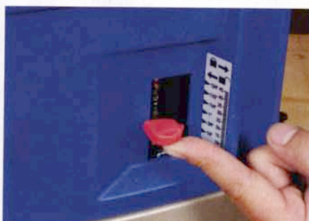
This neat device presets the finished height in 5mm increments from 5 to 45mm
