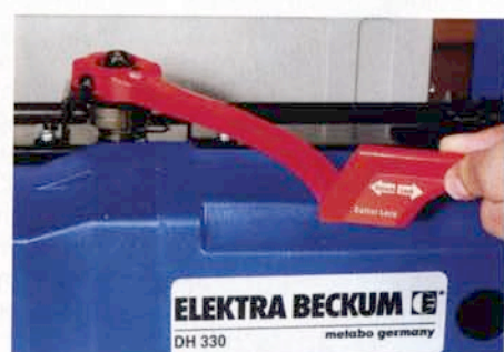
Locking the head keeps the cut uniform, although the thicknesser did show some snipe
