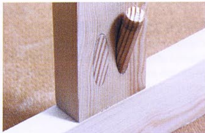
T-joint with plugs: one projecting, one sanded smooth
