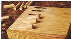
Glue the plugs into their pre-drilled holes
