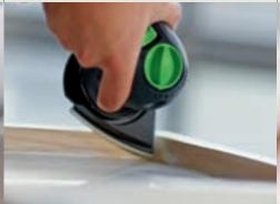
Save on costs: the tips of the sanding pad and abrasive can be used three times simply by rotating.
