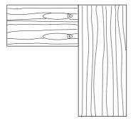
**Mitred Frame Corner Joints** – for narrow frames a single pocket hole is necessary. Cut the mitre and rout any rebates before boring the pocket holes. For material less than 50mm wide it may be necessary to tilt the pocket hole piece so that the hole is not perpendicular to the mitred edge.
