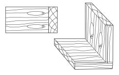
**T- Joints** – faster and stronger than dowel and biscuits. Self clamping whilst glue is drying.
