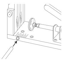
Push the support/end stop on from the other end of the bar through the hole in the side of the support.
