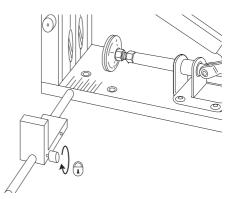
Place your workpiece onto the jig and adjust the end stops into position at the ends of the workpiece.
