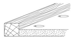
**Jig making** – very useful for jig making and temporary assembly operations. Ideal for routing jigs.
