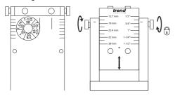
Turn the depth turret stop until the desired size is at the bottom of the bush.
