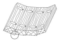
**Mitred Corner Joints** – joining two pieces with 45° mitres with the pocket jig is not advisable, however a 90° change of direction can be created by using a bevel-jointing piece. The joint comprises of a 90° infill piece with 45° mitres on both sides.
