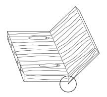
Pocket holes Angled Support Bare Board **Curved Joints** – this uses the same technique as the angled joint, but the angles will be shallower ( $5^{\circ}$  to  $15^{\circ}$ ). The overhang will need to be removed as previous.
