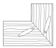
**Square Corner Joints** – faster and stronger than dowel and biscuits. Self clamping whilst glue is drying.
