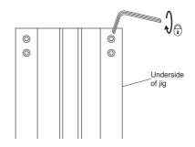
To remove the guide columns undo the guide column fixing screws.
