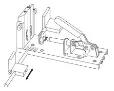
The built in push-pull clamp allows both hands to be free for drilling in both applications.
