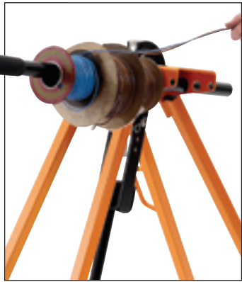
Using the extension and stabilising bar a cable reel feed can be created.
