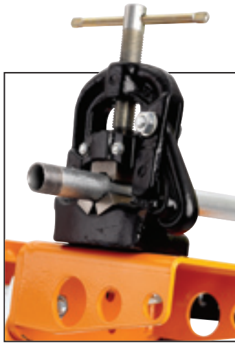
Vice can be secured over the edge of the mount to allow easy threading.
