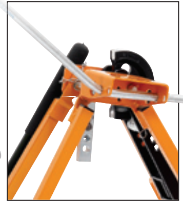
Pipes bends can be easily tweaked using the substantial vice mount.
