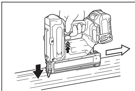
If the head of the nail remains above the workpiece surface, drive the nail while holding the nailer head firmly against the workpiece.
