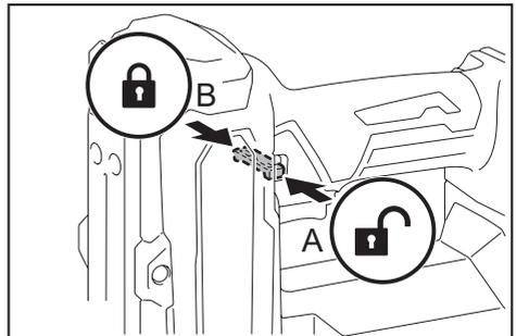
To prevent the switch trigger from accidentally pulled, the trigger-lock button is provided.
