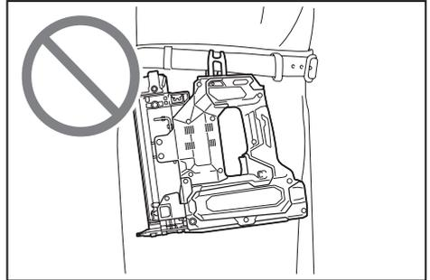
The hook is convenient for temporarily hanging the tool. This can be installed on either side of the tool.
