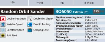
Standard Equipment : Abrasive disc, Dust nozzle, Side grip, Pad protector
