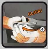
Push back the lever until you hear the click. Secure the lever with the security spring. The blade is now safely in position
