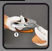
Hold the handle horizontally and pull the lever.
