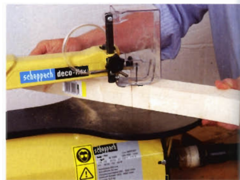
Cutting curves in 50mm thick softwood to see if it would be cut at 90°
