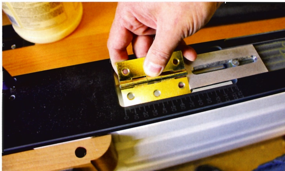
▲ Length is sorted by moving another stop to the hinge leaf
