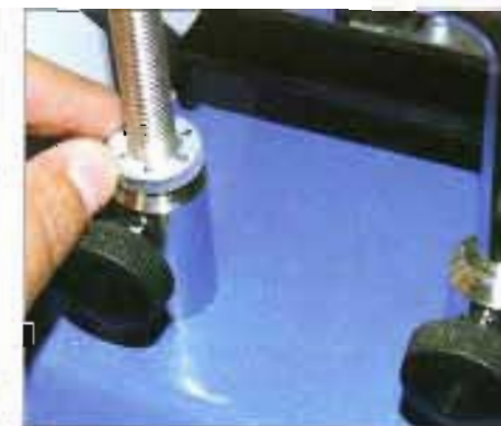
▲ Pic.3 ...while this wheel is used to micro-adjust the height of the tool post when setting the bevel angle
