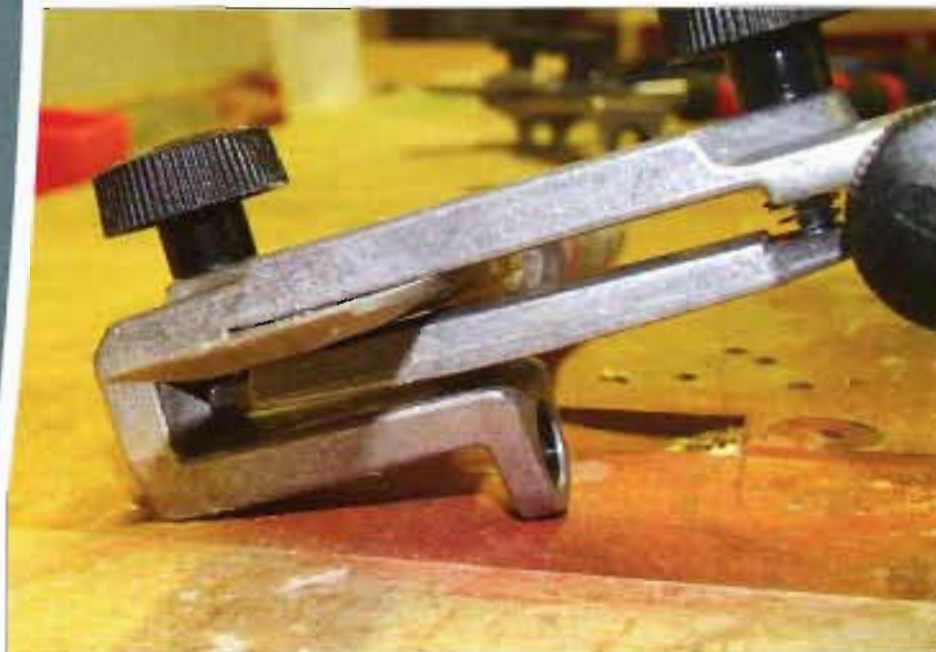
▲ Pic.1 The new tool clamp registers on the back of the tool so it stays square to the wheel at all times. The old clamp registered on the back so bevel tools could twist slightly and grind out of square
