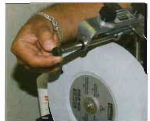
▲ Pic.4 A small screw-in knob stops the tool clamp from running off the tool post as you grind
