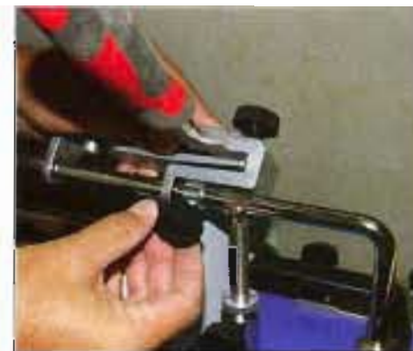
▲ Pic.2 This collar can be used to restrict the travel across the stone to stop it slipping off the edge...
