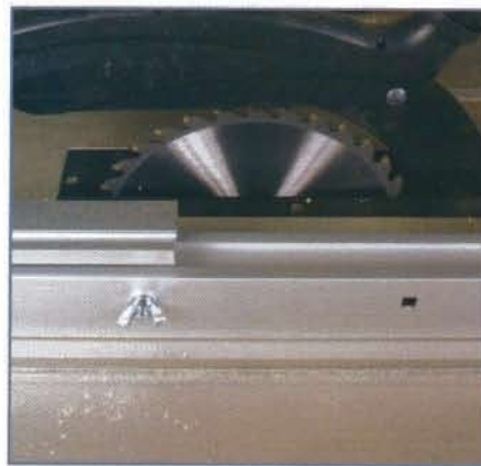
The rip fence cannot be drawn back far enough for ripping
