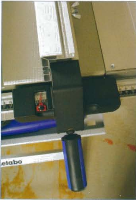
Clear scale reading and positive fence locking
