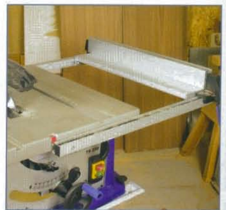
The table extension allows wide panel cutting
