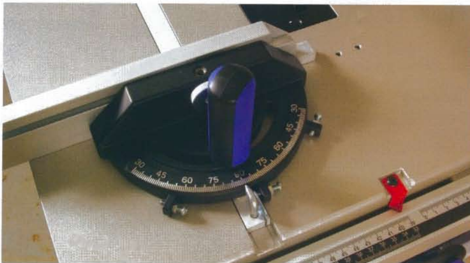
The protractor can be finely adjusted for accurate cutting
