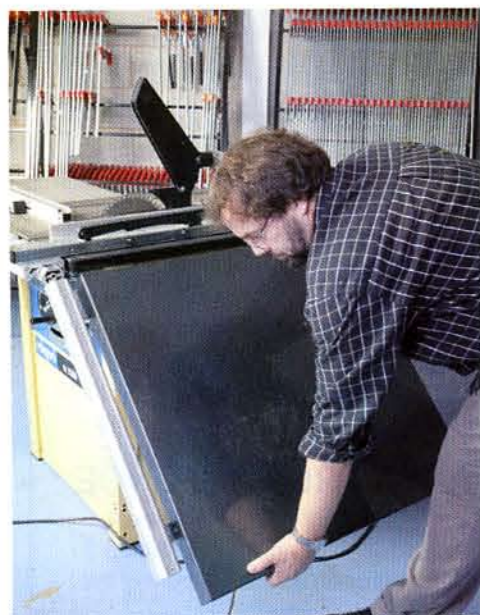
A hinged side table folds neatly out of the way after use, great for the space challenged workshop
