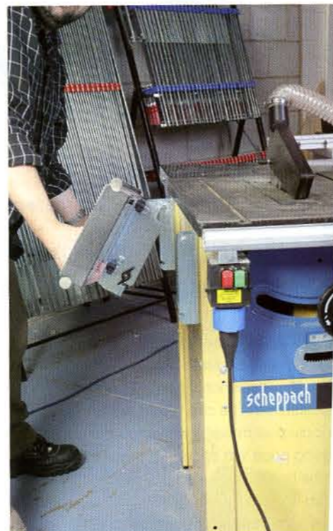
The sliding crosscut carriage hooks on the side of the machine
