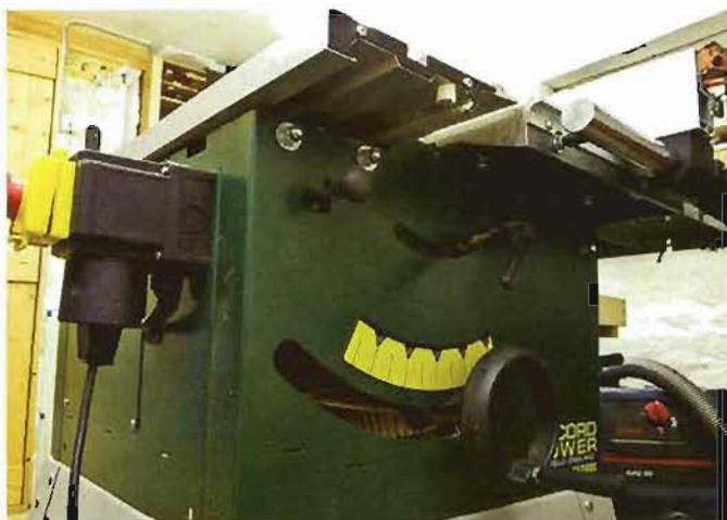
The saw body is of fabricated steel
