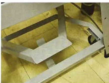
The foot locking pedal raises the saw bench onto wheels
