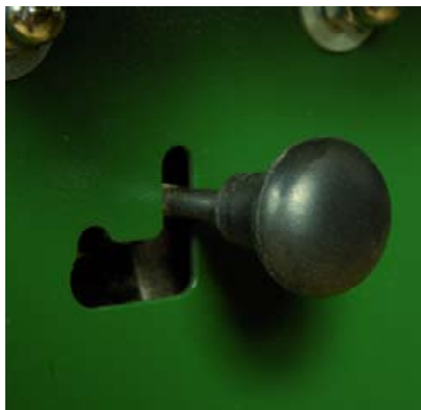
The sliding table lock is a nice touch and works well
