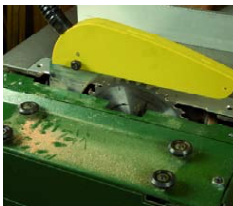
Blade changing is accessed by sliding the table off – note the wheels
