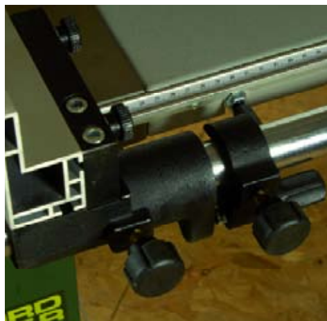
The fence is mounted on a strong round bar and the fine adjuster is simple but effective
