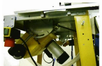
A clamp to the quadrant on each side locks the pivoting motor and blade guard box assembly at the chosen angle
