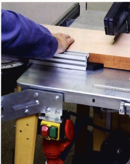
Crosscutting hardwoods is quick and clean on the 315mm blade running at 4000rpm
