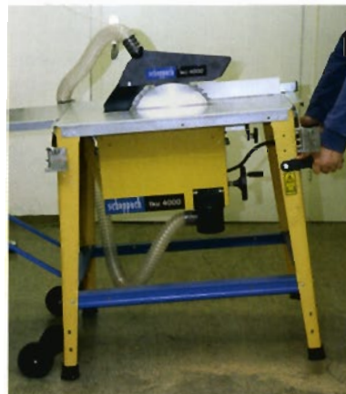
The 60kg saw is light enough to wheel around a workshop floor with ease
