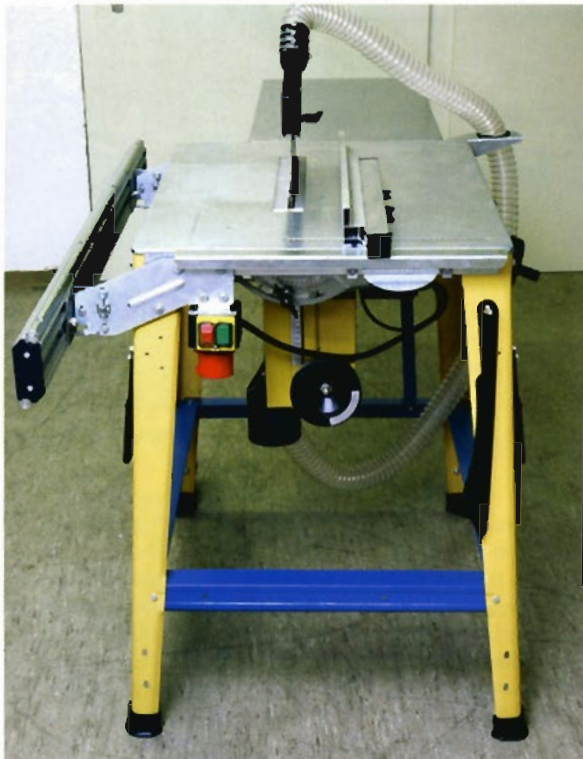
The tku4000 consists of an open steel frame with a steel tabletop and tilting motor unit slung beneath
