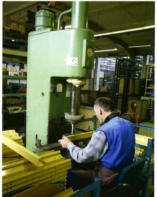
Built at Scheppach's factory in southern Germany, the main components are folded from laser-cut steel sheet which is powder coated
