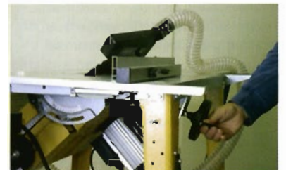
A hand-wheel beneath the right side of the table tilts the blade between -2° to the left and +45° to the right
