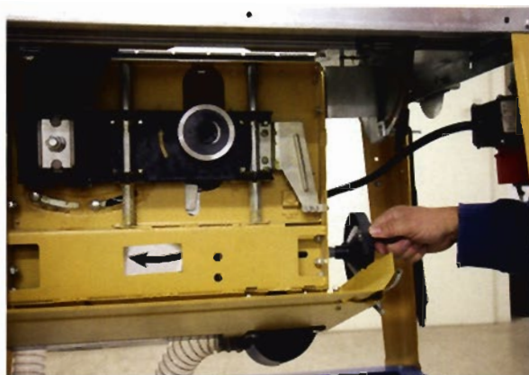
Height adjustment beneath the front of the machine moves the blade arbor up and down a pair of parallel rails
