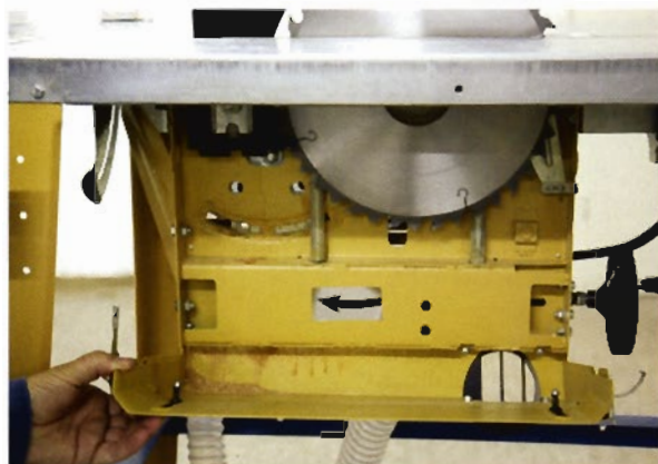
The blade guard box hinges down giving access to clear any sawdust blockage or change the blade
