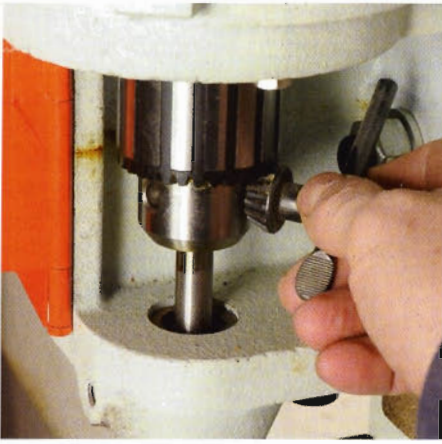
The chuck is a conventional keyed variety
