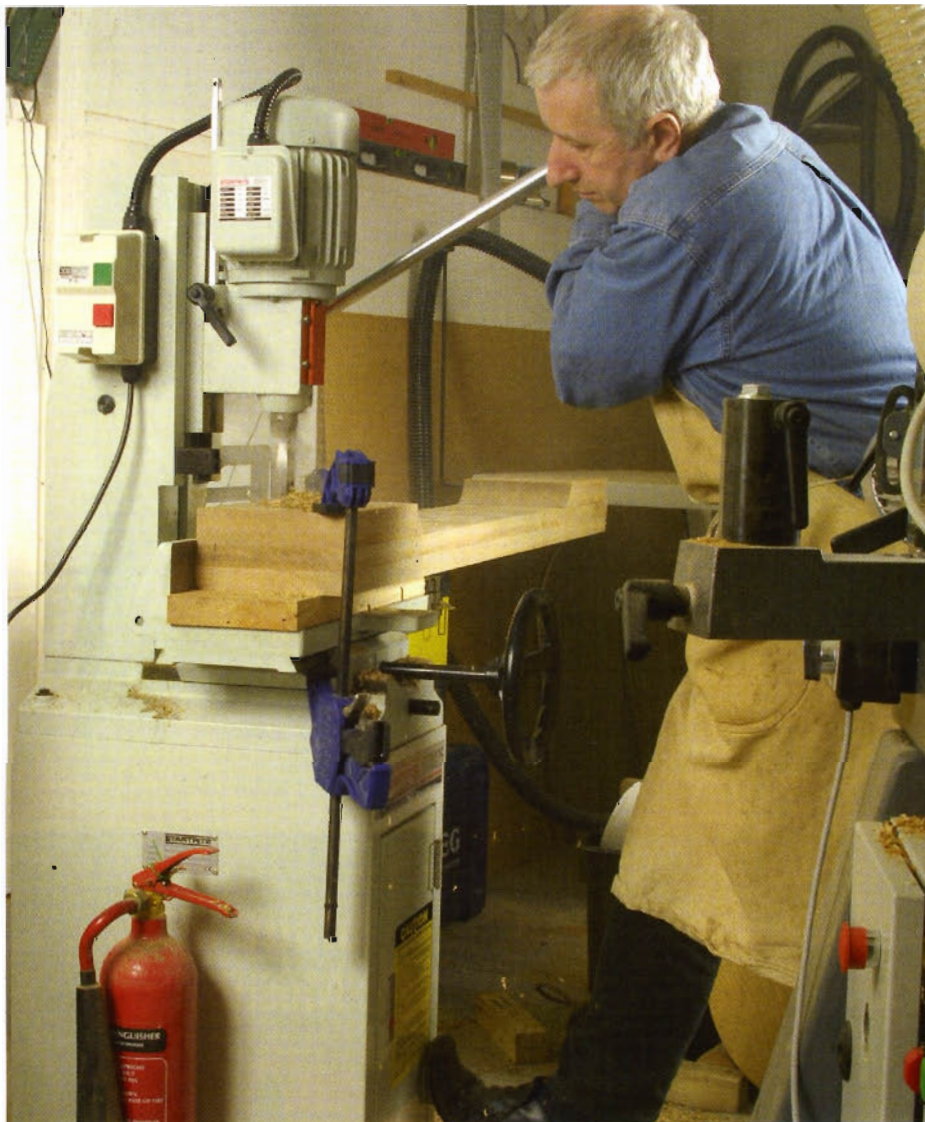
A bit of welly is required when cutting large mortises
