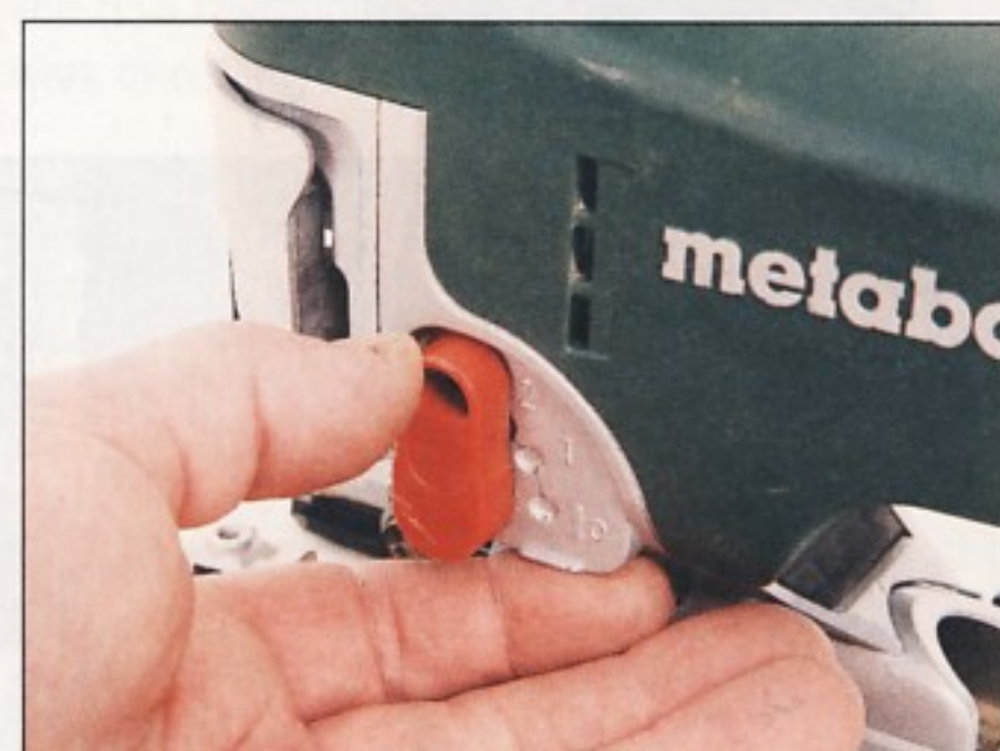
A four-position switch allows you to select the orbital action you require
