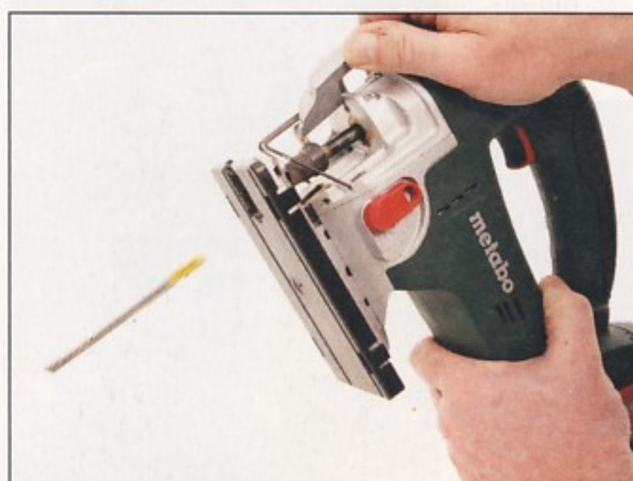
The quick ejection system shoots the blade out after use; just watch where it lands
