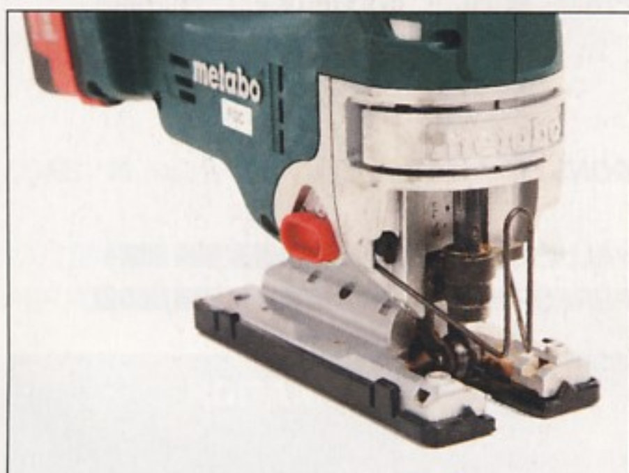
The diecast aluminium gearbox housing looks extremely solid and robust
