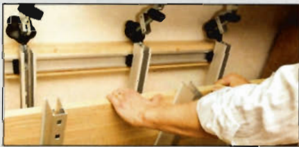
The vertical cramps fit onto a horizontal guide rail
