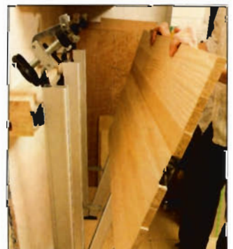
Releasing the cramps frees the assembled workpiece
