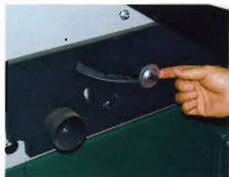
▲ Pic 3: These cogged plastic adjusters at the front and rear set the angle
