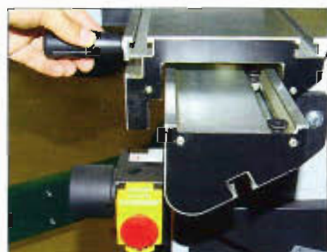
▲ Pic 1: The sliding carriage runs very smoothly, giving you a 900mm capacity...
