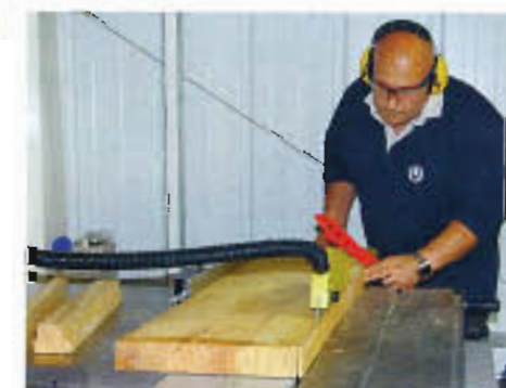
▲ Pic 6: Cutting 50mm-thick stock is easy, the blade leaving a clean finish
