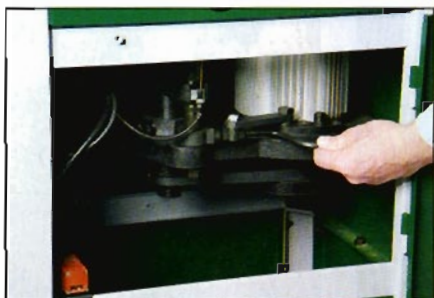
The motor is cleverly hinge-mounted to facilitate easy speed changes
