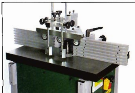
The guard has rollers for the overhead part – always an excellent arrangement
