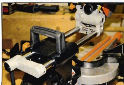
The handle at the back is useful for lifting the saw out.
