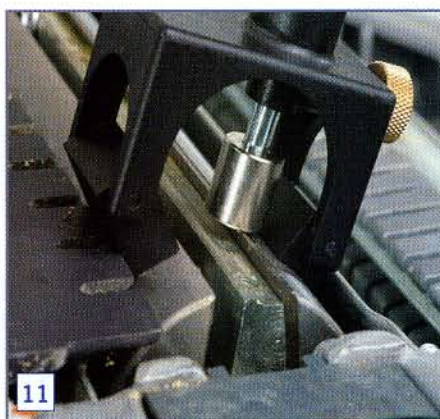
11 If you don't hve the setting data, zero the jig with an existing knife in situ, and lock up the setting rod
