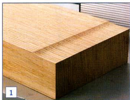
1 If the knives are set even a tad too high you'll get a snipe of the end of the board...
