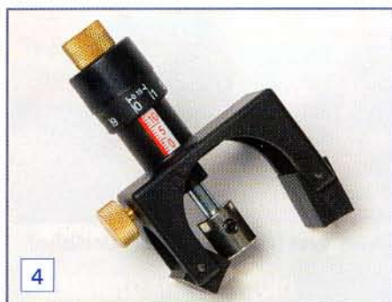
4 It comprises two magnetic jigs with micro adjustments on the central setting rod
