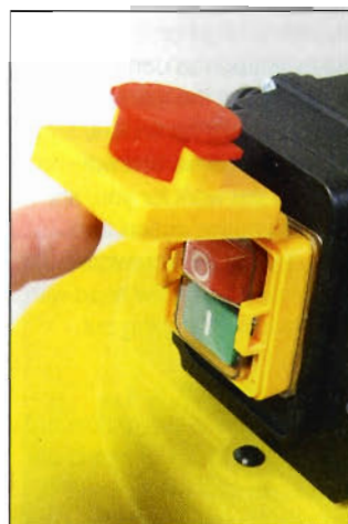
The shielded NVR switch on the motor body
