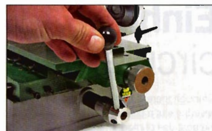
A single lever effects side-to-side movement
