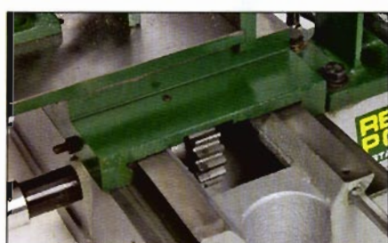
The table is moved by a large rack and pinion
