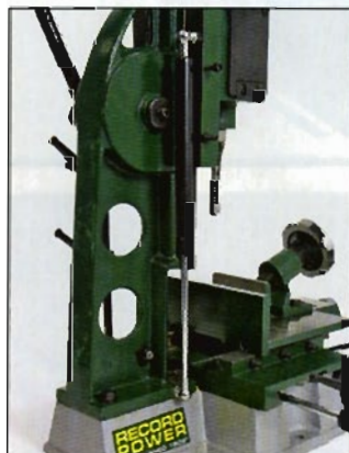
The machine is based around a substantial casting
