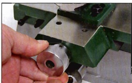
A small knob controls fore-and-aft movement
