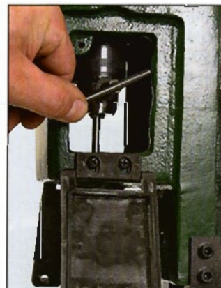
It's easier to tighten the chuck with the key vertical
