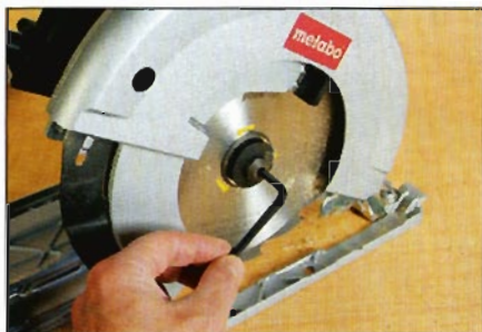
Changing blades is easy thanks to the spindle lock and supplied Allen key
