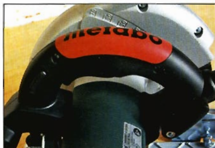
The main handle is rubber-insulated and houses the large power trigger
