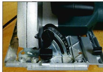
The cast magnesium baseplate can be set to any bevel angle up to 45°
