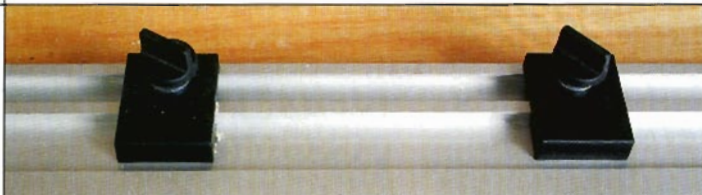
Adjustable stop blocks can be set to restrict the saw's travel along the rail
