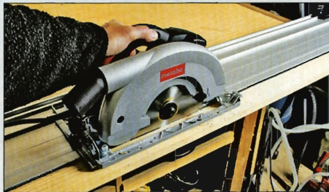
The saw sits on the guide rail with the blade running against its plastic edging strip
