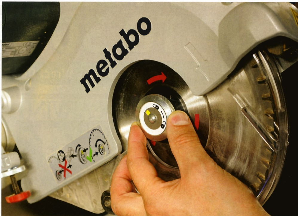
The toolless blade lock is unique so new users would benefit from a demonstration
