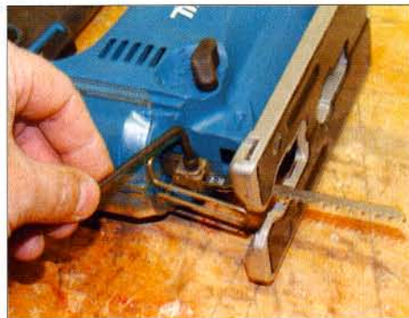
▲ Pic 2: Blade changing is done with the hex wrench, which stores on the body of the saw
