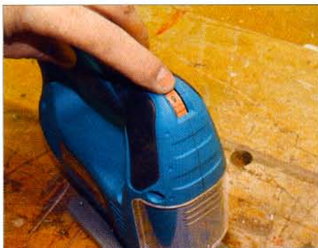
▲ Pic 1: The speed adjuster wheel is basic, but easy to alter as you cut
