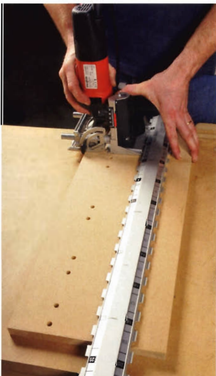
Drilling template for large panel work
