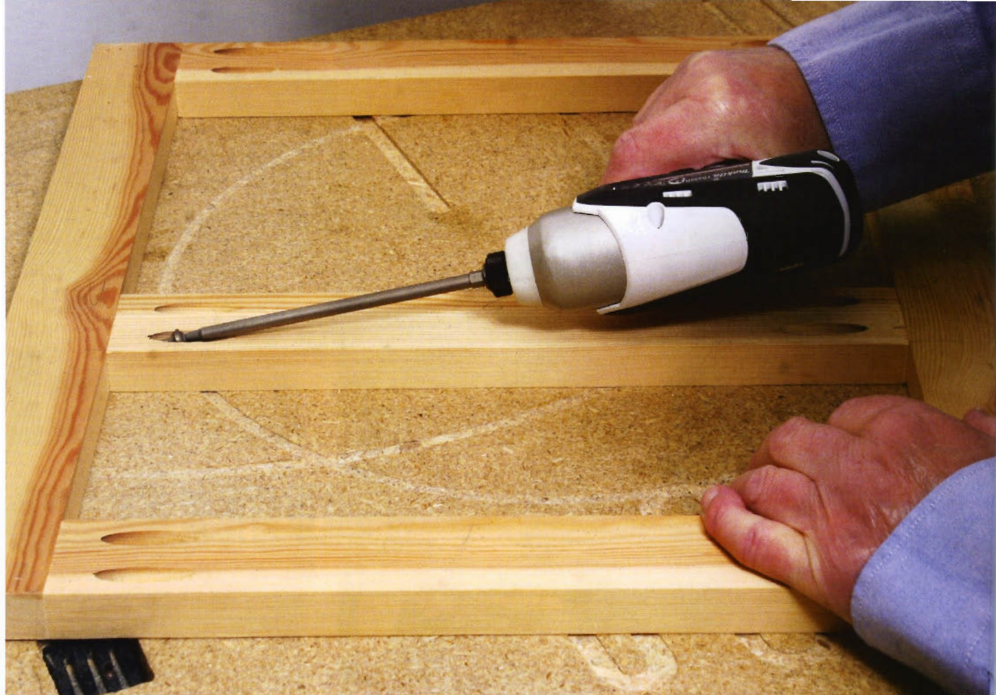
Dismantling a pocket-holed frame with the impact driver
