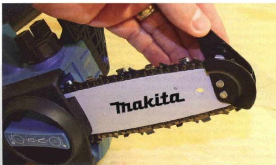
▲ Pic.3 This nose guard is riveted on to prevent plunge cuts and possible kickback
