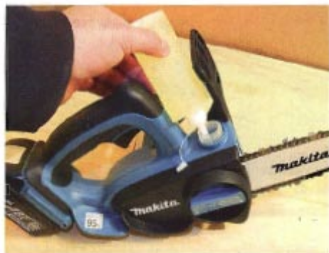
▲ Pic.1 You need to apply chain oil to the reservoir but after that it's self lubricating
