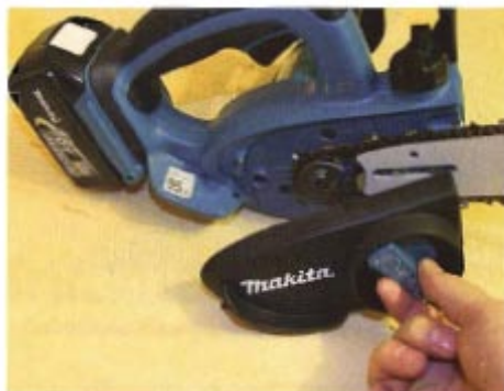
▲ Pic.2 Swapping chains is simple, the cover simply unscrews with the large dial knob
