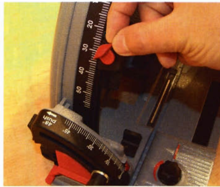
▲ Pic.2 Rotating this button automatically compensates for the thickness of the guide rail – pretty nifty
