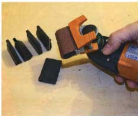
▲ Pic. 4 These rubber sanding blocks are ideal for cleaning up intricate mouldings
