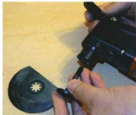
▲ Pic. 2 The accessories are clamped with the serrated post held with the cam lock
