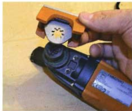
▲ Pic. 3 The star profile lets any accessory swing to the best position to suit the work
