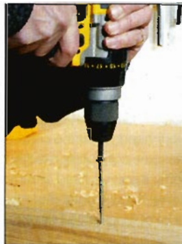
The slowest speed provides ample power for driving large screws
