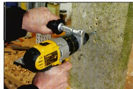
With hammer action activated, masonry drilling is fast and efficient
