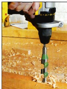
The self-tightening chuck increases its grip as you use the tool
