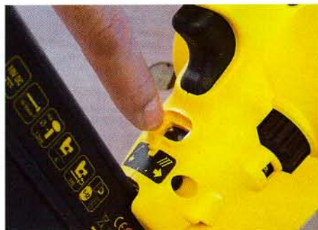
▲ Pic 4: Flipping this switch puts the gun into 'bump' mode for fast nailing
