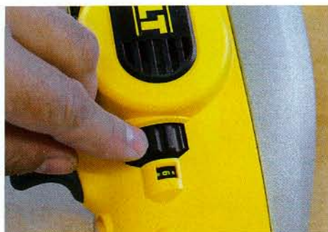
▲ Pic 3: The click-stop dial with which the depth of drive is set is a bit stiff but works well
