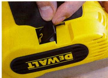
▲ Pic 2: Flipping this lever locks the gun to prevent it from firing
