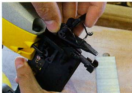
▲ Pic 1: Jammed fixings are easily freed thanks to this toggle clip nose
