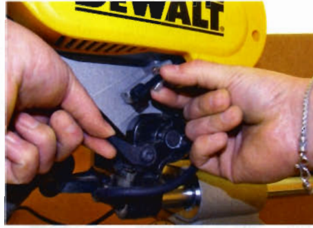
▲ Pic.2 This flip stop is easily altered for different trenching depths
