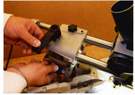
▲ Pic.3 These levers are used to tilt and lock the saw for compound work. The lower one is pretty stiff
