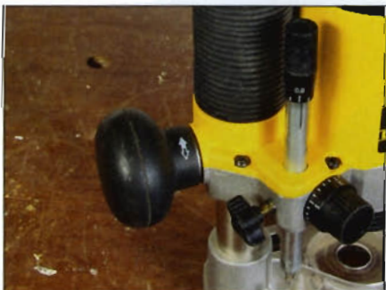
The rack-and-pinion depth of cut
