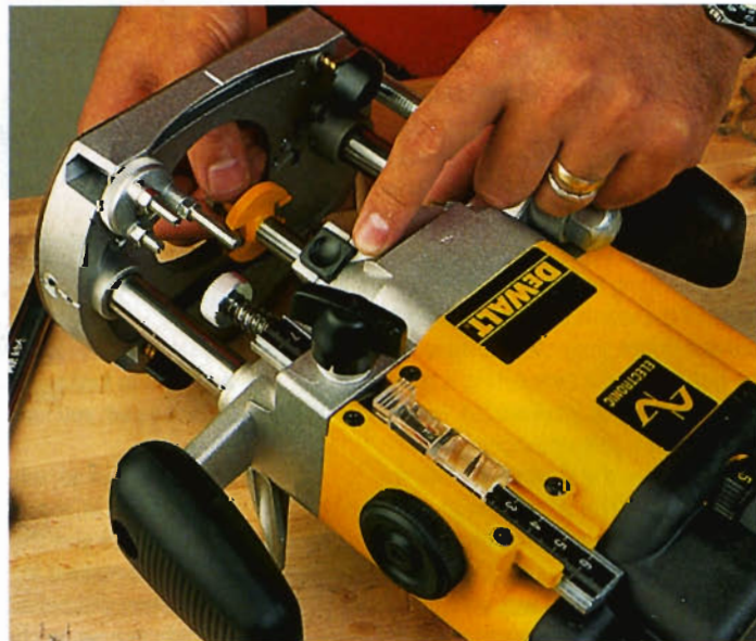
▲ Pic.2 As standard, a spindle lock button is used to swap cutters
