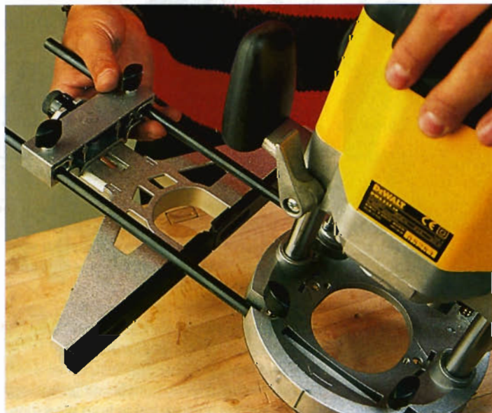
▲ Pic.1 The micro adjustable fence is still one of the best on the market
