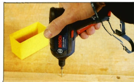
A squeeze of the trigger selects first gear to drive the screw home
