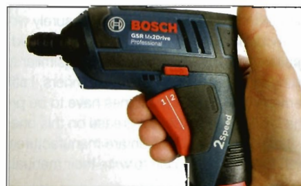
The ingenious speed selector is incorporated into the trigger
