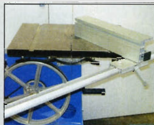
The front rail swings clear for blade changing
