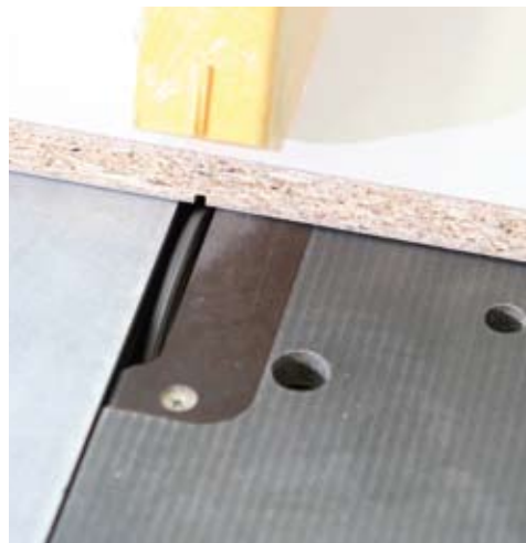
Split scoring blade can be set to the perfect cutting width and height.
