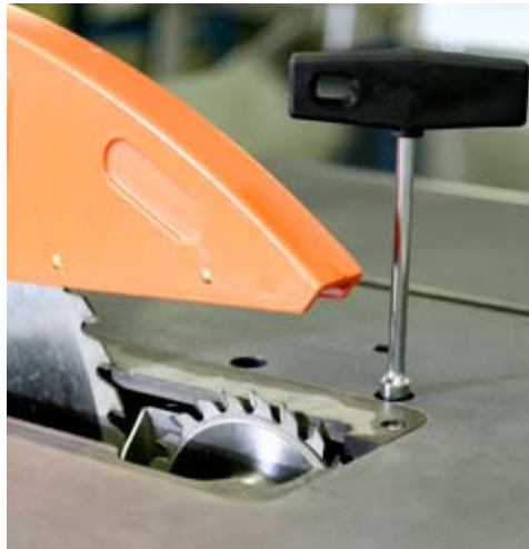
Positive adjustment of the scoring blade for both height & lateral movement
