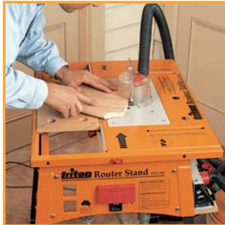
Safe free-hand operation when safety guard is fitted on its own to the table top
