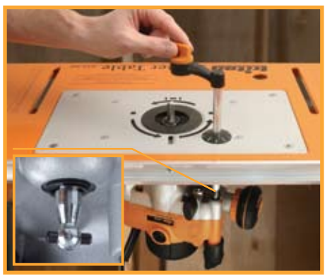
Top of table height adjustment is possible using the height winder handle from the TGA150 template guide kit
