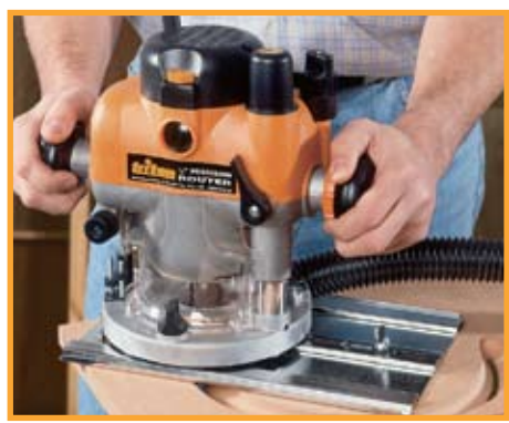
Multi-function fence provides excellent control for hand-held use and circle cutting
