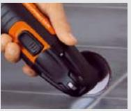
Where tile joints have to be removed and regrouted, the round diamond saw blade is the economic solution, both in terms of time saved and blade life.
