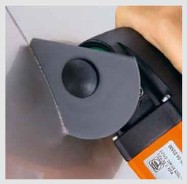
Cut sheet steel and plastics up to a max. 19 gauge (1 mm) thick with the HSS segment blades, burr-free and non-warping, with a minimum of flying sparks – without complicated touch-up work. Can also be used universally in corners.
