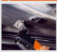
Even stubborn undercoatings can be removed easily with the rigid scraper blade in the fastest possible time.
