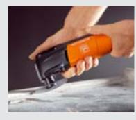
Brittle puttied edges can be removed without any problem and without any danger of glass breakage.
