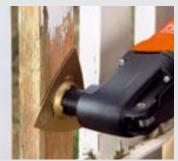
With the carbide rasp, remove stubborn signs of weathering thoroughly and quickly thanks to the high sanding capacity.
