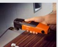
With the E-CUT saw blades, trim plasterboard and make cut-outs easily for electrical installations etc. in sheets that have already been installed.
