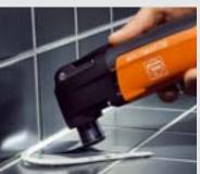
The flexible scraper blade is perfect for removing elastic materials, such as caulking, adhesive residues or paint
