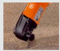
Cut rigid material such as plastic or carpet simply and without any problems with the convex segment blade.
